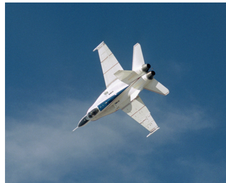
NASA Dryden Flight Research Center Photo Collection http://www.dfrc.nasa.gov/Gallery/Photo/index.html NASA Photo: EC04-0361-16 Date: December 15, 2004 Photo By: Carla Thomas NASA's flexible-wing F/A-18 maneuvers through a test point during the second phase of the NASA/Air Force Active Aeroelastic Wing flight research program.
