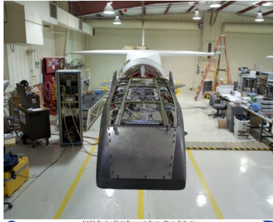
NASA Dryden Flight Research Center Photo Collection http://www.dfrc.nasa.gov/gallery/photos/index.html NASA Photo: EC01-2019-20 PSD Date: January 22, 2001 Photo by: Tom Tachida Head-on view showing the X-43A hypersonic research aircraft after it was mated to its modified Pegasus® booster rocket.
