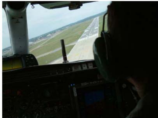
c) Correction to centerline
